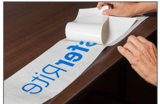
Peel the paper backing away from the graphic to ensure successful transfer.
